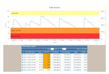
The Hall Effect sensor reading, along with the geometry of the tank, are used to calculate the fill level of the liquid in the tank, which is displayed on the Xact website. This lets you access tank fill levels, historical readings, GPS location, ambient temperature, and other critical data points to optimize your delivery planning.
